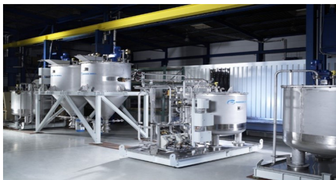
Decontamination - Plant for the decontamination of metal waste. Source Bilfinger (left), Cyclife Sweden (right)
