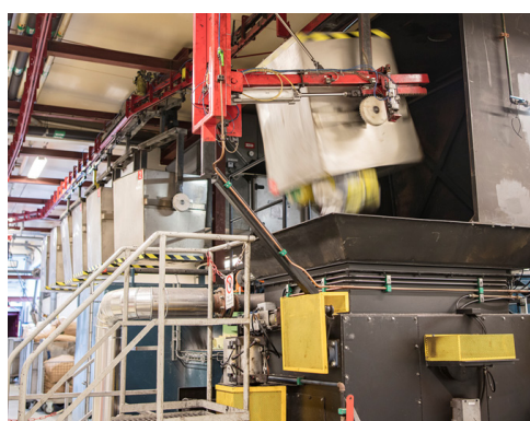
Volume reduction – Melting and incineration. Source: Cyclife France/Cyclife Sweden
