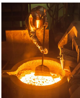
Volume reduction – Melting and incineration. Source: Cyclife France/Cyclife Sweden
