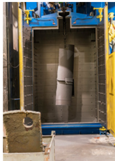
Decontamination - Plant for the decontamination of metal waste. Source Bilfinger (left), Cyclife Sweden (right)
